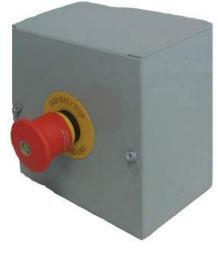
Height: 101.6 mm (4 in) Diameter (Ø): 45 mm (1.77 in) Length: 48 mm (1.89 in) 1.36 kg (3 lbs) Surface-mount, Type 1 (IP 20 equivalent) 1 N.C. (Normally Closed) Screw clamp 4-20 AWG stranded, 14-18 AWG solid Switch: UL Listed, CSA Certified, CE Marking, IEC 60947-5-1 Enclosure: UL Listed, CSA Certified
